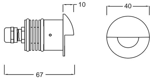
Los is a wall recessed floor washer luminaire ideal for paths and stairs illumination. Constructed from Inox 316 with a heat sink assembly, O-rings and a first fix sleeve ensures a long lasting fixture and watertight seal. The deep recessed led position and the 5mm clear safety glass ensures anti-glare efficiently and creates visual comfort. IP67 rating as standard makes Los suitable for both indoor and outdoor residential, public-buildings applications.
