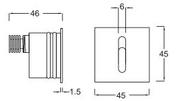
Bambu-T is a wall recessed floor washer luminaire ideal for paths and stairs illumination. Specially designed with a deep angled lens shield to produce a soft asymmetric light emission. Constructed from aluminium and O-rings to ensure a long lasting fixture and maximum protection. Mounting box is needed for installation.
