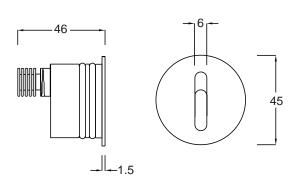
Bambu is a wall recessed floor washer luminaire ideal for paths and stairs illumination. Specially designed with a deep angled lens shield to produce a soft asymmetric light emission. Constructed from aluminium and O-rings to ensure a long lasting fixture and maximum protection. Mounting box is needed for installation.
