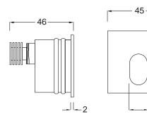
Ogi T is a wall recessed floor washer luminaire ideal for paths and stairs illumination. Specially designed with a deep angled lens shield to produce a soft asymmetric light emission. Constructed from aluminium and O-rings to ensure a long lasting fixture and maximum protection. Mounting box is needed for installation.
