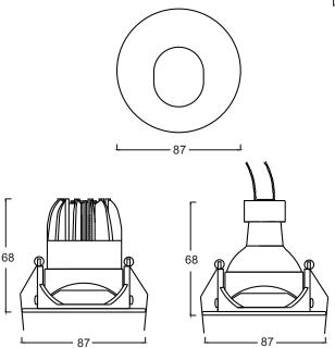
Anesis flush the ceiling downlight supplied with a separate die cast aluminium-kit for seamless appearance in plaster ceilings.
