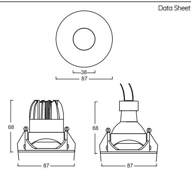
Anesis pinhole flush the ceiling downlight with Ø 38mm pinhole aperture and supplied with a separate die cast aluminium-kit for seamless appearance in plaster ceilings. Available in both white or black finish as standard.
